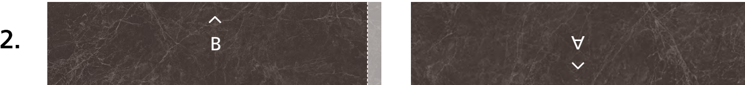
Rotate part A 180°. Plan to join parts A & B for continuation of the main veins and remove the surplus.
