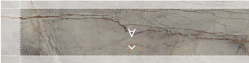
Rotate part A 180°. Plan to join parts A & B for continuation of the main vein and remove the surplus.
